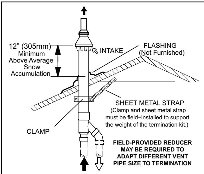
**Figure 35. Direct Vent Concentric Rooftop Termination**
