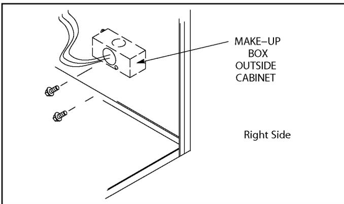
**Figure 56. Exterior Make-Up Box (Field Provided Right Side)**
