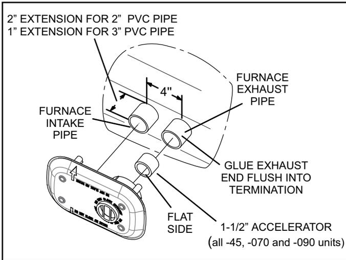
**Figure 34. Flush Mount Side Wall Termination**
