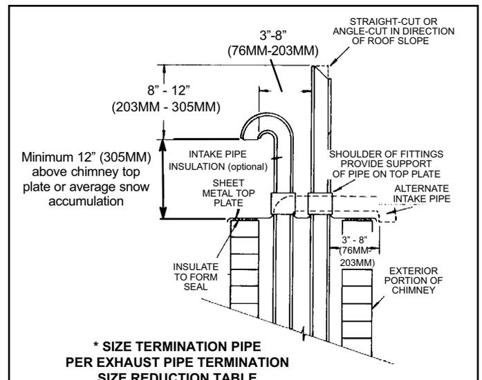
**Figure 38. Direct Vent Application Using Existing Chimney**
