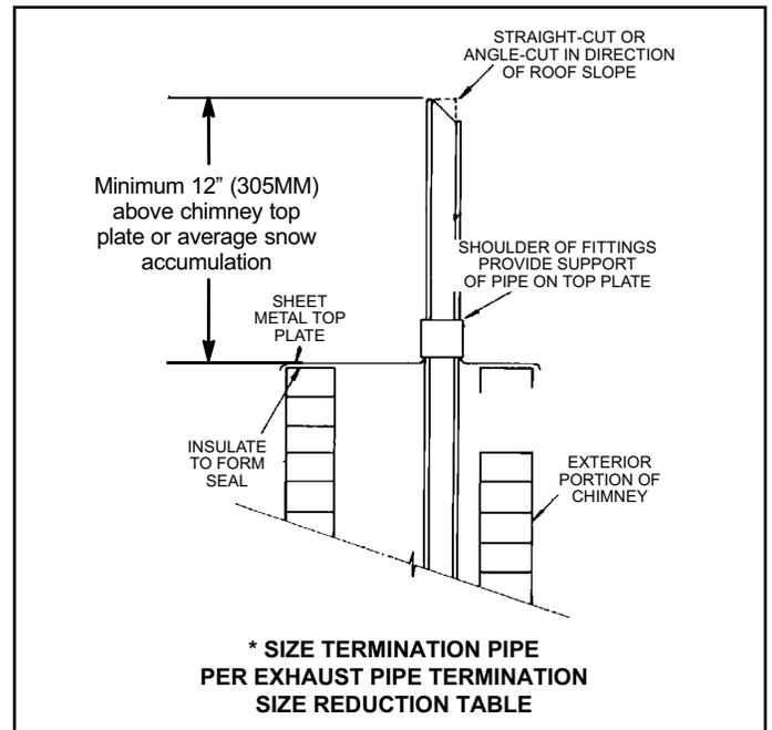
Figure 43. Non-Direct Vent Application Using Existing Chimney
