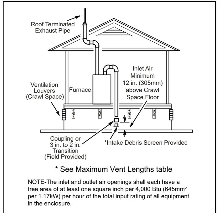
**Figure 27. Equipment in Confined Space
