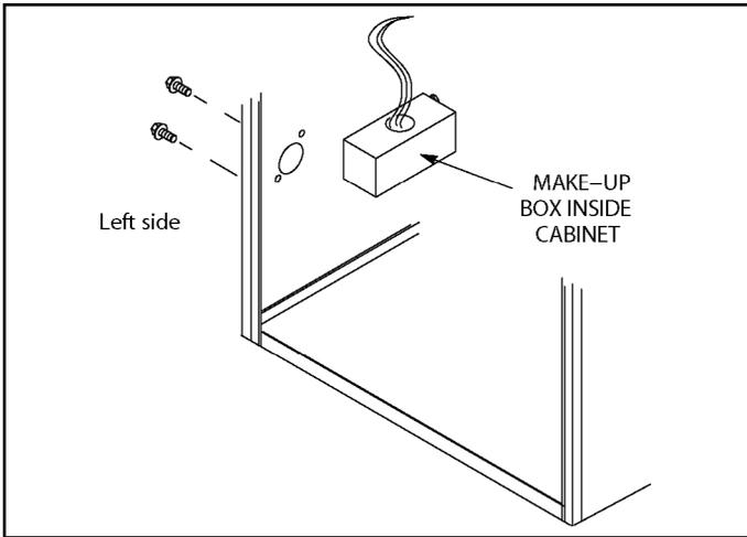
**Figure 55. Interior Make-Up Box (Factory - Installed Left Side)**
