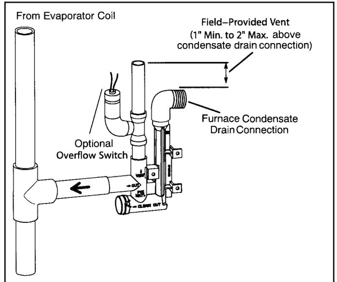
**Figure 51. Condensate Trap with Optional Overflow Switch**
