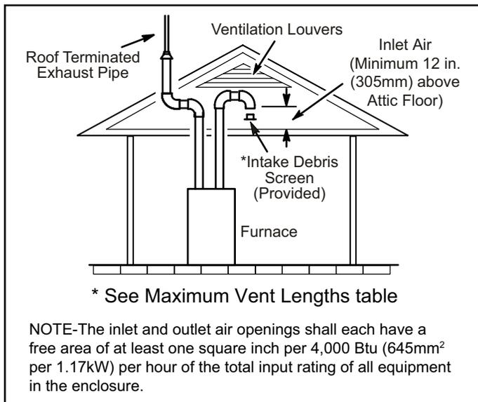
**Figure 26. Equipment in Confined Space
