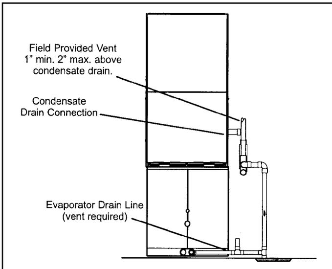
**Figure 50. Evaporator Coil Using a Common Drain**
