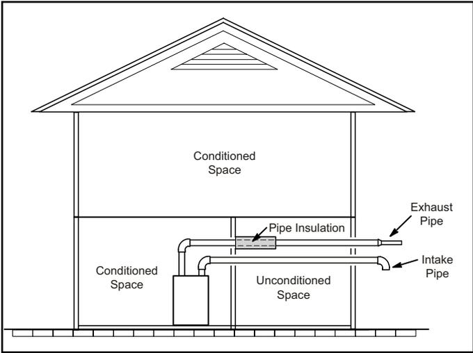
**Figure 28. Insulating Exhaust Pipe in an Unconditioned Space**
