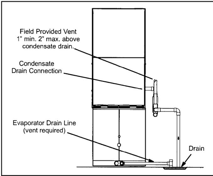
**Figure 49. Evaporator Coil Using a Separate Drain**
