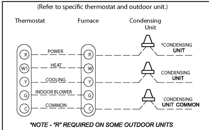
**Figure 57. Furnace and Condensing Unit Thermostat Designations**
